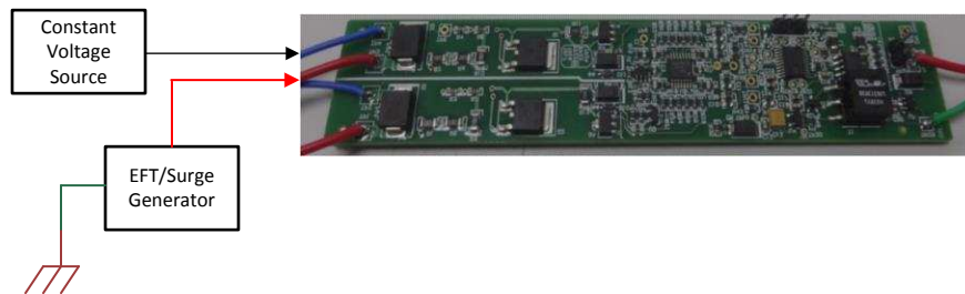
図 18. EFT Setup for Binary Input Module With BI Digital Isolator
