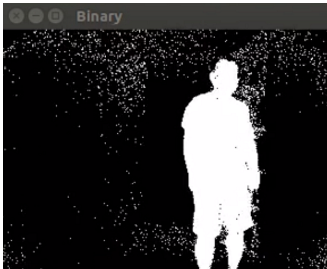
☒ 10. Background Subtraction Binary Image
