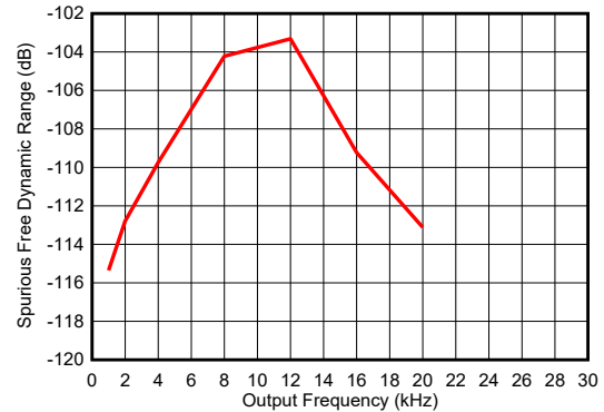
DAC update rate = 768 kHz, V_{REFPF} = 4.5\text{ V} , V_{REFNF} = -4.5\text{ V} , sixth-order, low-pass, 30-kHz output filter
