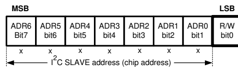
Figure 16. I 2 C Chip Address (0x2C)
