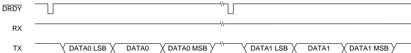
Figure 65. Automatic Data Read Mode (Continuous Conversion Mode)
