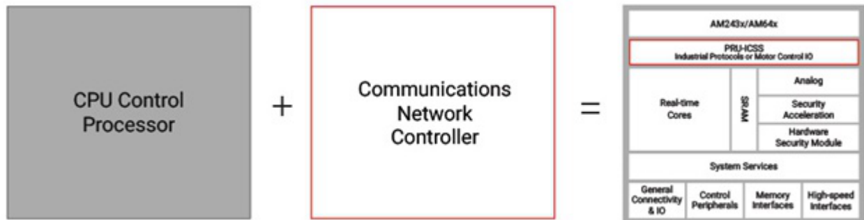
Figure 2. The PRU-ICSS in Both the AM64 MPU and AM243 MCU Families Provides a Single-chip Solution for Real-time Control and Communications
