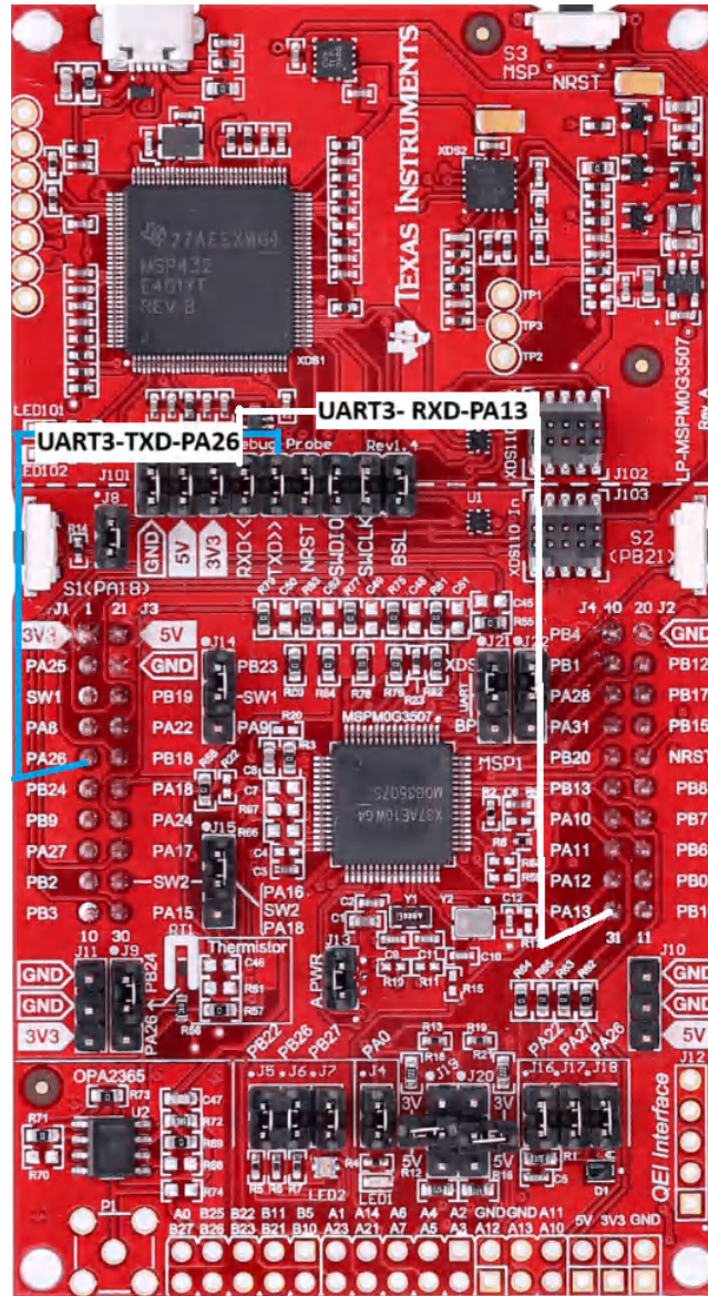
Figure 2-5. LP-MSPM0G3507 Backchannel Connection to UART3 [As UART 3 port is used for serial communication in DRV8316 Project]
