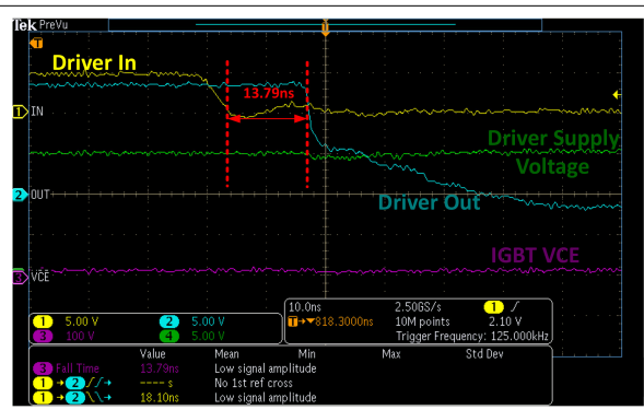
8-3. UCC27524A-Q1 Used to Drive IGBT in the Boost Converter
