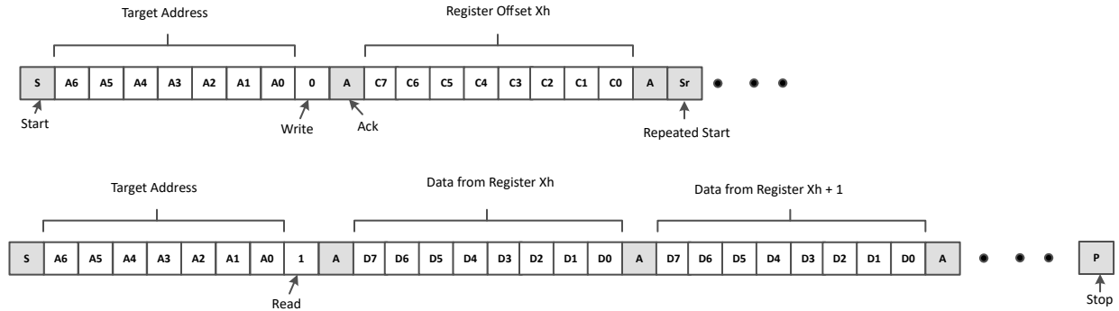
図 6-4. I2C Read With Repeated Start
