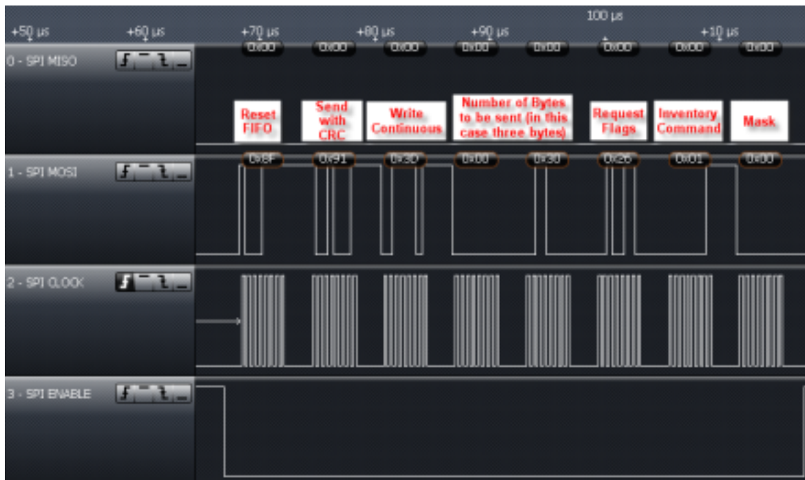
Figure 6-22. Inventory Command Sent From MCU to TRF7964A
