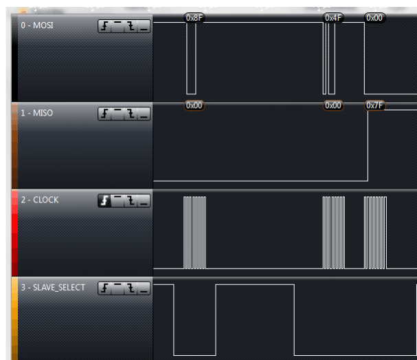
Figure 6-26. Reset FIFO and Read RSSI
