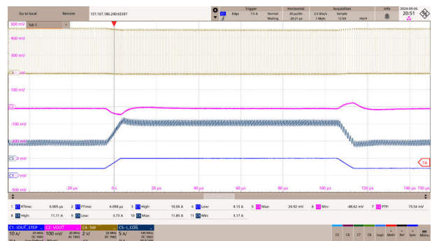
9-31. Load Transient - PFM Operation
