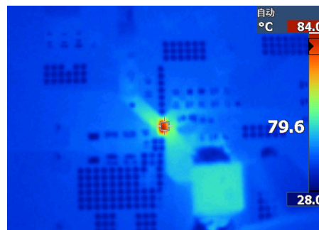
图 8-7. Case Temperature, V_{IN} = 24\text{ V} , I_{OUT} = 3\text{ A} , f_{sw} = 500\text{ kHz}
