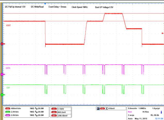
Figure 13. PMBus 1-MHz Bus Speed with 1.8-V Pullup
