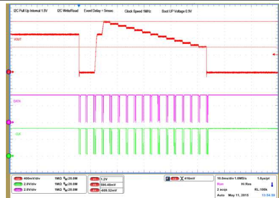
Figure 16. 6 Sequenced Events – I2C Write/Read with PEC
