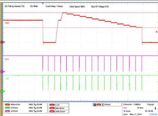
Figure 15. 6 Sequenced Events – I2C Write/Read
