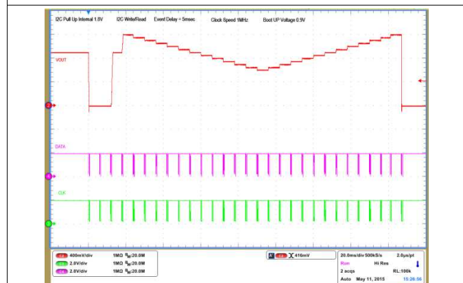
Figure 19. 17 Sequenced Events – I2C Write/Read with PEC
