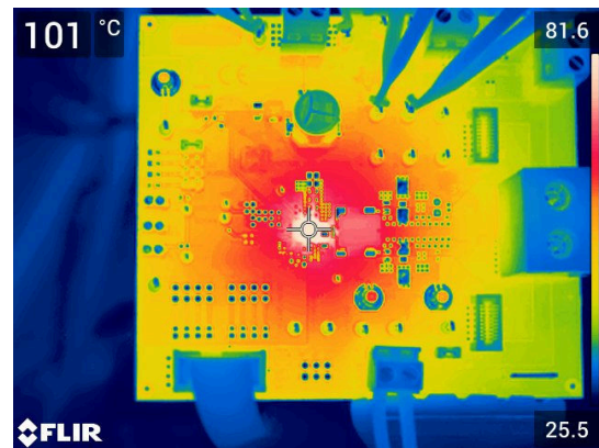
8-26. Thermal Characteristics, 1.2-MHz FCCM, External 5-V Bias, 35-A Load
