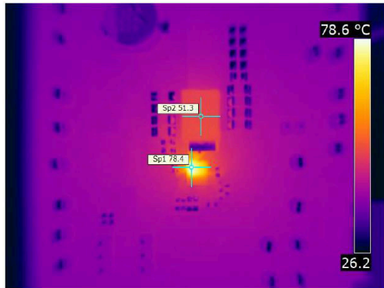
图 6-13. Thermal Image at 15-A Output Current
