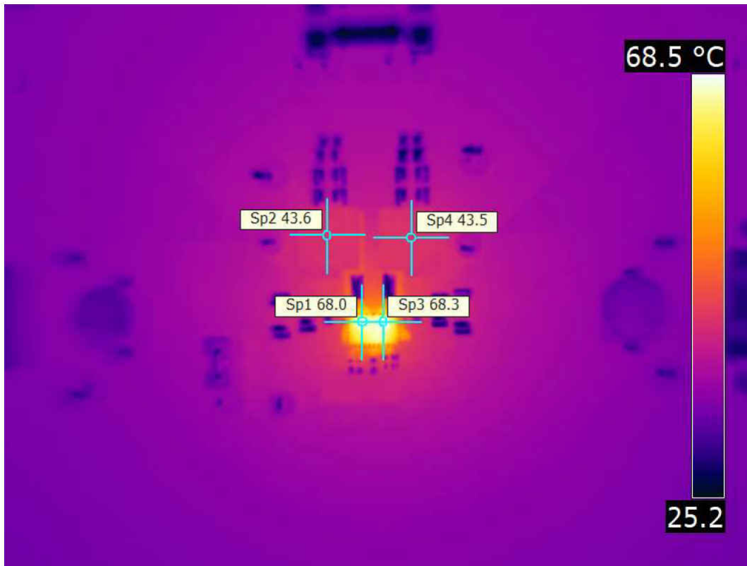
☒ 10-3. Thermal Image at 25°C Ambient - 2-phase Operation, f_{sw} = 1 MHz, V_{IN} = 12 V, V_{OUT} = 1 V, I_{OUT} = 12 A, Inductor = 560 nH (3.3 mΩ typical)
