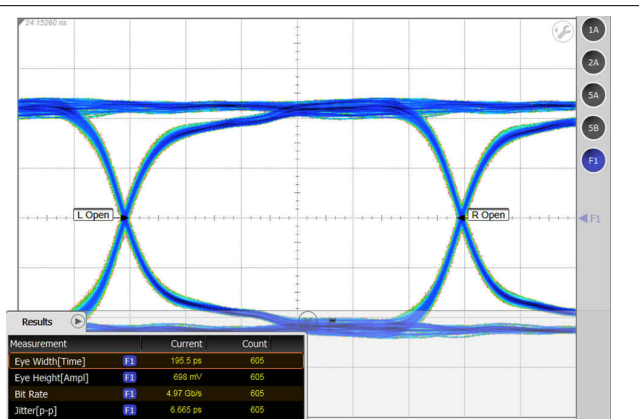
9-4. 5 Gbps PRBS-7 Signals Through a Typical TMUXHS4212 Channel in TI Evaluation Board
