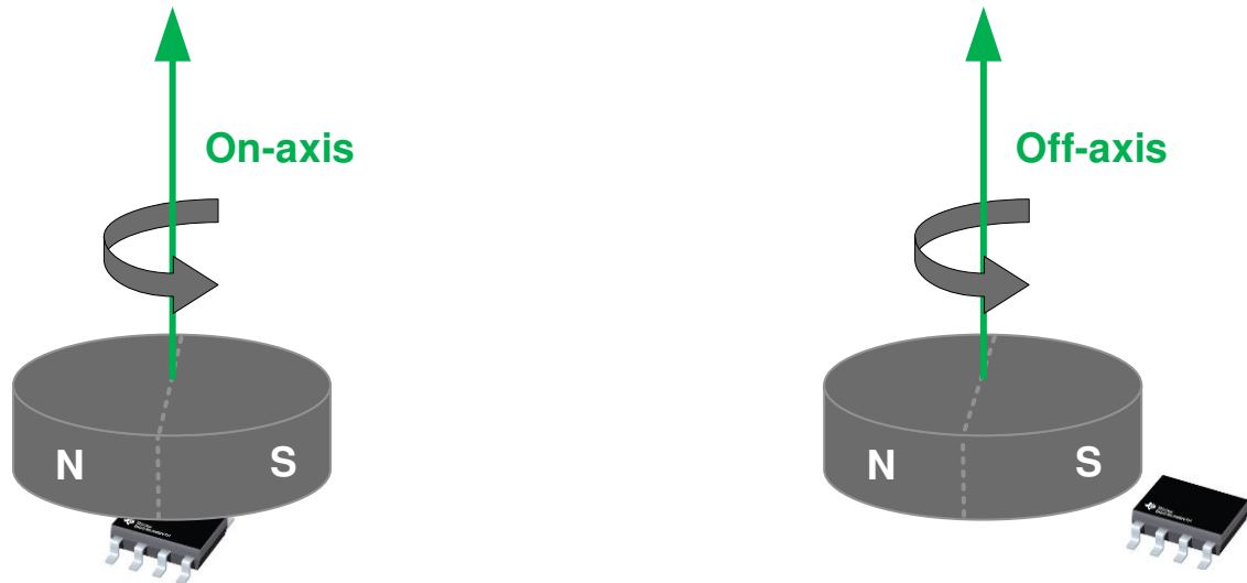
图 8-5. On-Axis vs. Off-Axis Angle Measurements
