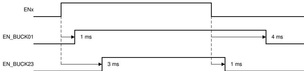
图 10. Typical Start-Up and Shutdown Sequencing
