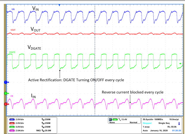
10-4. AC Super Imposed Test - 2-V Peak-Peak 30 KHz
