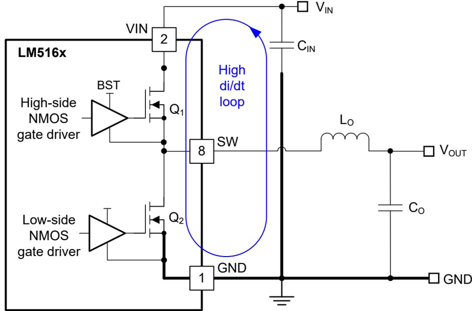
**図 8-40. Critical Current Loops in the Buck Converter**
