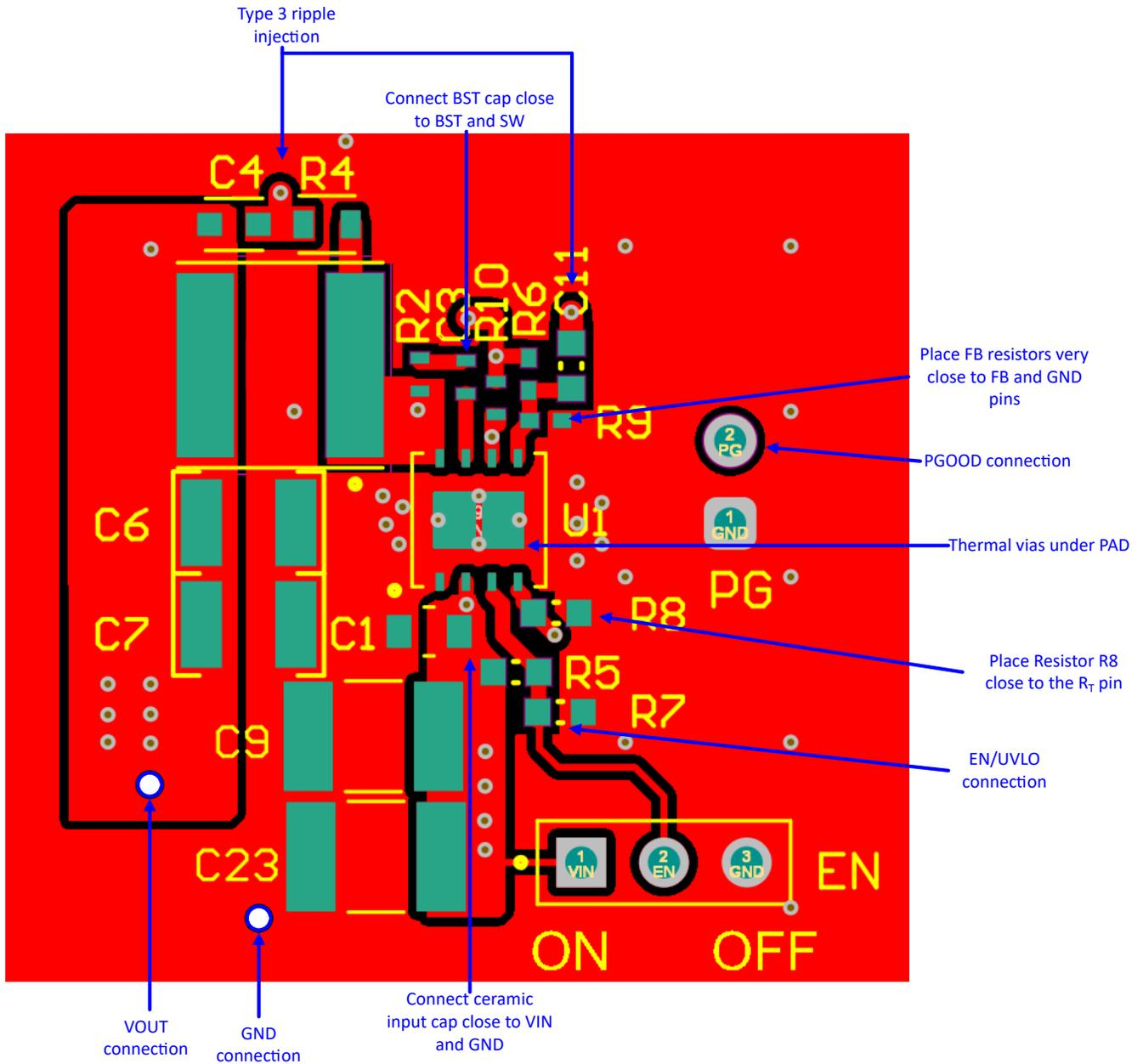
図 8-42. LM516x PCB Layout Example for NGU package
