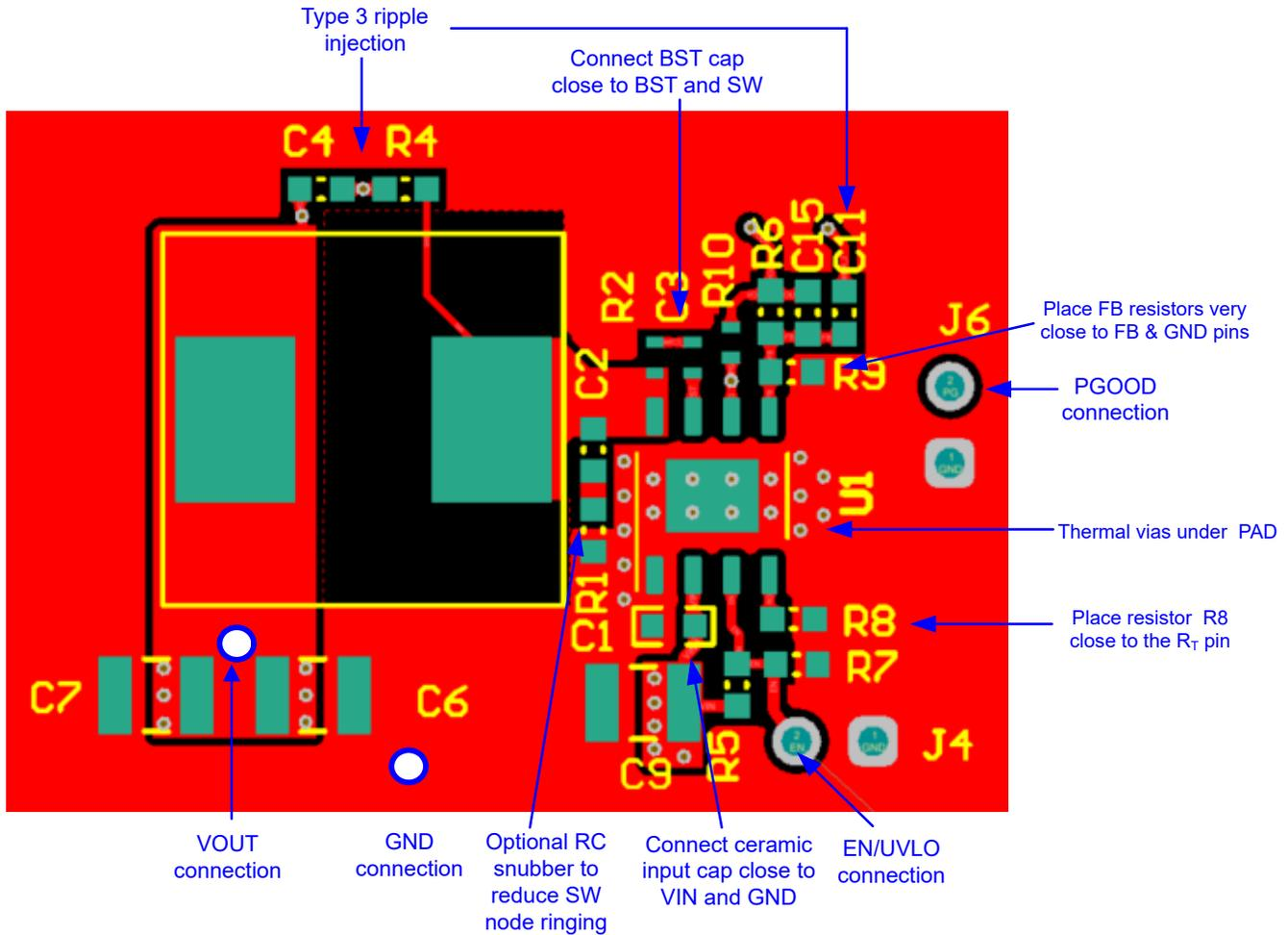
Figure 8-41. LM516x PCB Layout Example for DDA package
