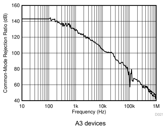
6-11. Common-Mode Rejection Ratio vs. Frequency
