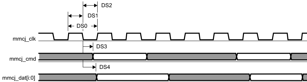
图 5-100. MMC/SD/SDIOj in - Default Speed - Transmitter Mode
