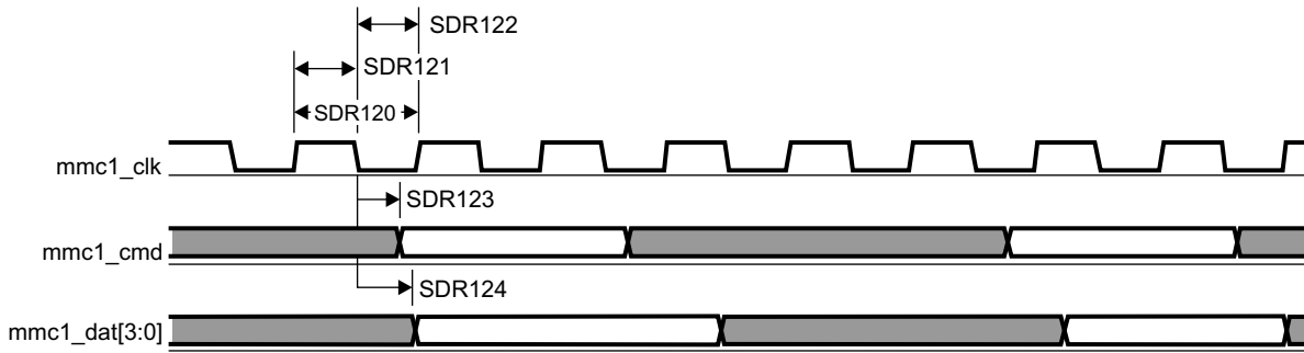
图 5-83. MMC/SD/SDIO in - High Speed SDR12 - Transmitter Mode
