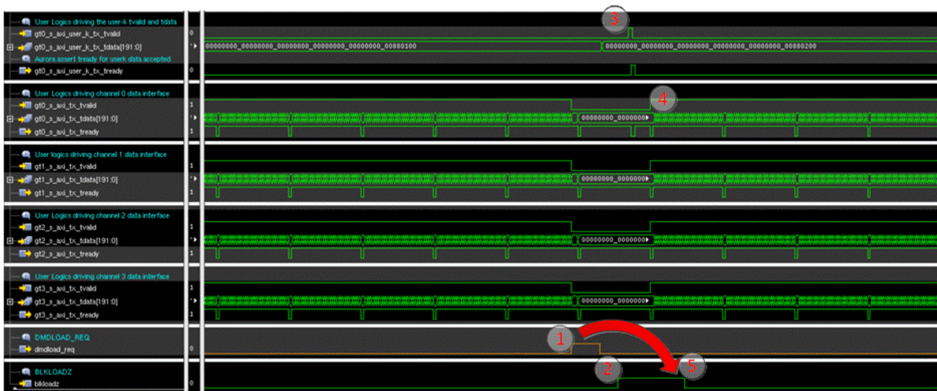
Figure 7-5. End of Block DMDLOAD_REQ Assertion Followed by New Block Control Word Waveform
