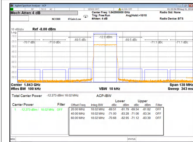
8-4. Dual band ACPR Performance in Downlink Band 3 with On-chip PLL
