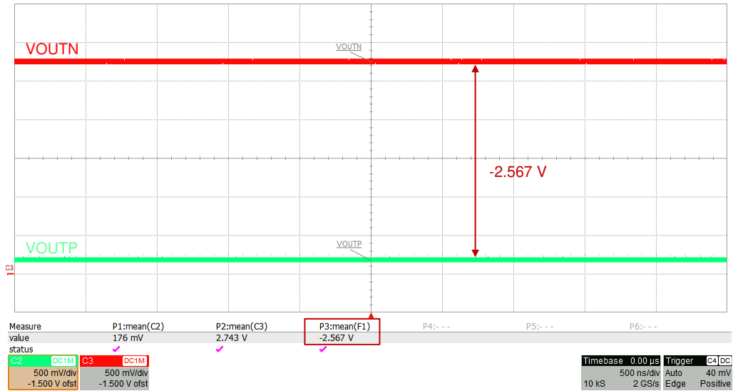
図 6-5. Typical Fail-Safe Output of the AMC3330-Q1
