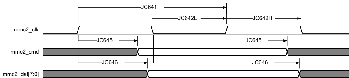
Figure 7-78. MMC/SD/SDIO in - High Speed JC64 - Transmitter Mode
