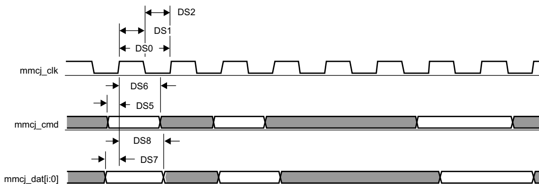
Figure 7-82. MMC/SD/SDIOj in - Default Speed - Receiver Mode
