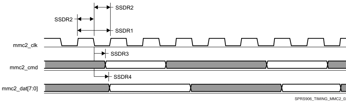
Figure 7-76. MMC/SD/SDIO in - Standard JC64 - Transmitter Mode
