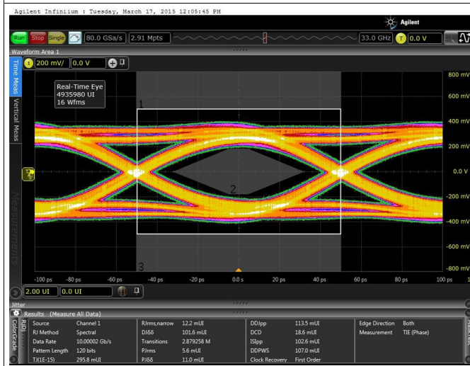
Figure 80. Eye Diagram at 10-Gbps Bit Rate with Default Output Swing
