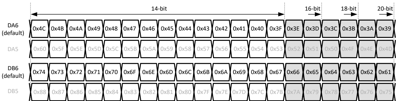
Figure 8-46. 1-wire output bit mapping
