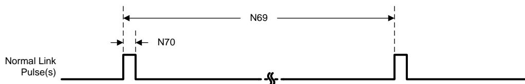
图 5-36. 10Base-TX Normal Link Pulse Timing
